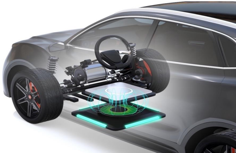
Figure 2- 15 Inductive type charging
